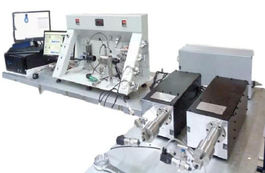
Figure 3. IFT-PDSA-02 apparatus which belongs to APEX Co. as a drop shape analysis equipment.
