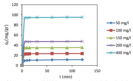
Figure 6. Effect of the contact time and initial dye concentration on BB159 adsorption by banana peel.
