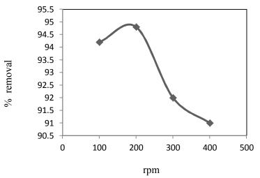
Figure 5. Effect of mixing speed on the adsorption of BB159 by banana peel.
