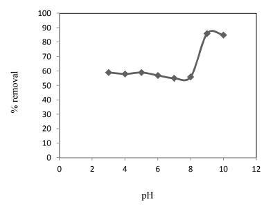
Figure 4. Effect of pH on the adsorption of BB159 by banana peel.
