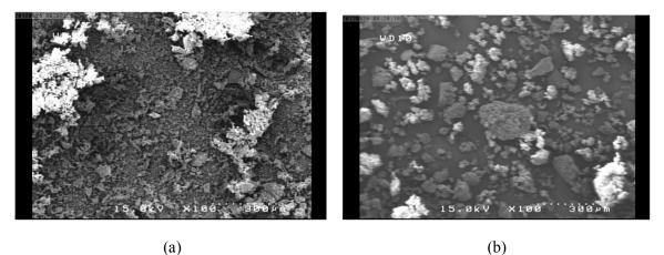
Figure 2. Field emission scanning electron microscope of (a) banana peel and (b) dye adsorbed banana peel.
