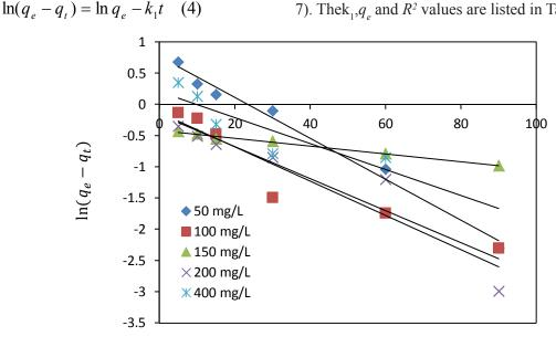
t(min) Figure 7. Pseudo first order kinetics for BB159 adsorption on banana peel.
