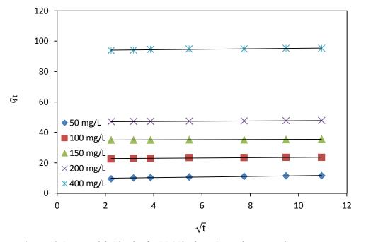
igure 10. Intra particle kinetics for BB159 adsorption on banana peel.
