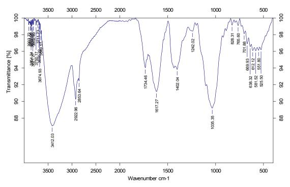
Figure 1. FTIR spectrum of banana peel.
