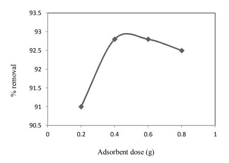
Figure 3. Effect of adsorbent dose on the adsorption of BB159 on banana peel.
