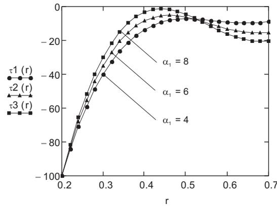
Fig. 2. Profiles of the shear stress  $\tau(r, t)$  given by Eq. (3.31) - curves  $\tau_1(r)$ ,  $\tau_2(r)$ ,  $\tau_3(r)$  for  $f = -1$ ,  $R_1 = 0.2$ ,  $R_2 = 0.7$ ,  $\nu = 0.0001637$ ,  $\rho = 880$ ,  $t = 10s$ ,  $\beta = 0.8$  and different values of  $\alpha_1$ .
