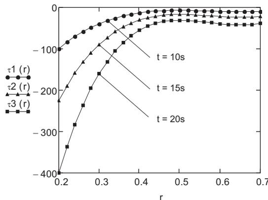
Fig. 1. Profiles of the shear stress  $\tau(r, t)$  given by Eq. (3.31) - curves  $\tau_1(r)$ ,  $\tau_2(r)$ ,  $\tau_3(r)$  for  $f = -1$ ,  $R_1 = 0.2$ ,  $R_2 = 0.7$ ,  $\nu = 0.0001637$ ,  $\rho = 880$ ,  $\alpha_1 = 5$ ,  $\beta = 0.8$  and different values of  $t$ .
