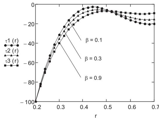
Fig. 3. Profiles of the shear stress  $\tau(r, t)$  given by Eq. (3.31) - curves  $\tau_1(r)$ ,  $\tau_2(r)$ ,  $\tau_3(r)$  for  $f = -1$ ,  $R_1 = 0.2$ ,  $R_2 = 0.7$ ,  $\nu = 0.0001637$ ,  $\rho = 880$ ,  $\alpha_1 = 5$ ,  $t = 10s$  and different values of  $\beta$ .
