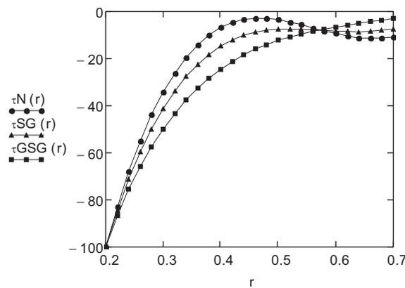
Fig. 4. Profiles of the shear stress  $\tau(r, t)$  given by Eq. (3.31) - curves  $\tau_1(r)$ ,  $\tau_2(r)$ ,  $\tau_3(r)$  for  $f = -1$ ,  $R_1 = 0.2$ ,  $R_2 = 0.7$ ,  $\nu = 0.0001637$ ,  $\rho = 880$ ,  $\alpha_1 = 5$ ,  $t = 10s$  and  $\beta = 0.8$ .
