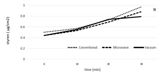
Fig. 2. The amount of migration in food stimulant water by different heating processes.
