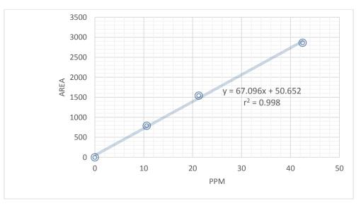
Fig. 1. The calibration curve indicating the acrylamide concentration against the area of the peak by HPLC
