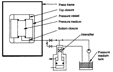
**Fig. 1.** A schematic of an indirect compression equipment for high pressure processing (After Mertens (1995).) (Fellows, 2000)
