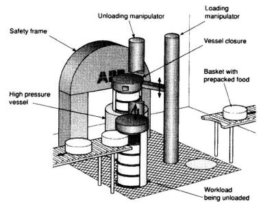
**Fig. 2.** A schematic drawing of a production unit for high pressure treatment at pressures between 400-800MPa (From Olsson (1995)) (Fellows, 2000)
