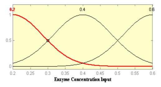
Fig. 3. Gaussian membership functions for input 1
