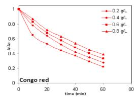
Fig. 4. Effect of the amount of C,N,S-tridoped  $SnO_2$  on the photodegradation efficiency Conditions: dye concentration=50 mg/L, pH= 6.5, V=50 mL.
