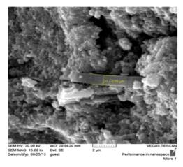
**Fig. 2.** SEM image of C,N,S-tridoped SnO<sub>2</sub> nanoparticles.
