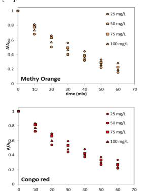
**Fig. 5**. Effect of initial dye concentration on the photodegradation efficiency Conditions: photocatalyst=0.4 g/L, pH= 6.5, V=50 mL.
