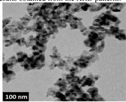
**Fig. 3.** TEM image of C,N,S-tridoped SnO<sub>2</sub> nanoparticle.
