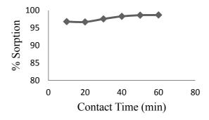
**Fig. 7.** Effect of contact time on the removal of MG by PAni/SD.
