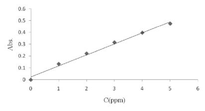
Fig. 3. Calibration curve of absorbance against oncentration of malachite green.
