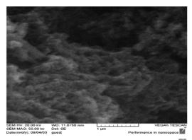
Fig.12. SEM picture from PAni/SD/MG.
