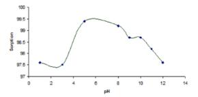
**Fig. 5.** Effect of solution pH on adsorption percentage of MG by PAni/SD.
