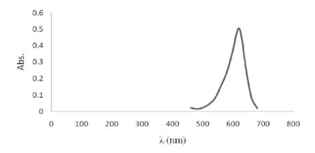
Fig. 4. Absorption spectrum of malachite green.
