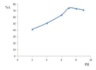
Fig. 3. The effect of initial pH of the solution on the adsorption percentage of  $Pb^{2+}$  ion onto nG (C<sub>o</sub>=20PPm, t<sub>c</sub>=50 min,T=298K, m<sub>nG</sub>=0.10g).
