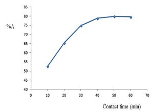
Fig. 1. The effect of contact time on the adsorption percentage of Pb2+ ion onto nG ( $C_o=20$ PPm, T=298K, pH=6, m<sub>nG</sub>=0.07g).
