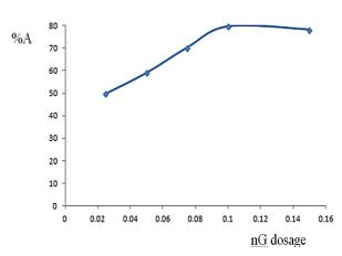
Fig. 2. The effect of nG dosage on the adsorption percentage of lead ion onto nG ( $C_0=20PPm$ , T=298K, pH=6, t<sub>c</sub>=50min).
