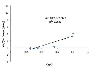
Fig. 9. BET plot for lead ion adsorption onto nG.
