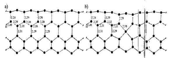
Fig. 1. The 2D views of (a) the pristine and (b) the defective models of SiNTs. The values of optimized bond lengths are written on the selected bonds.
