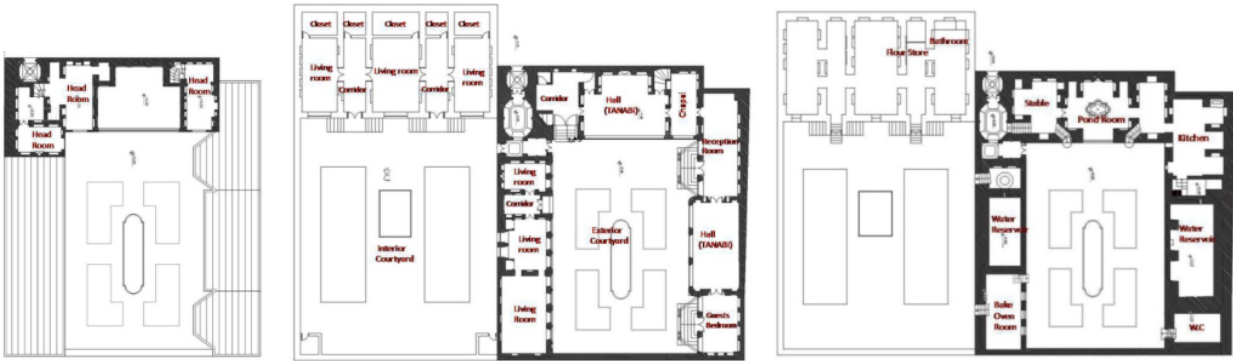
Fig.6: Plans of the Salmasi House complex, from right: basement, ground floor, first floor
