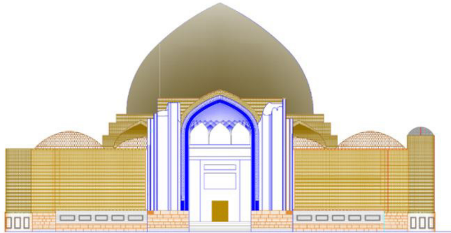
Fig.3 : The installation of stone blocks in the lower construction level to prevent the increasing humidity in the Blue Mosque (c. 1491) (Moradi & Houseinpour, 2018, 101).
