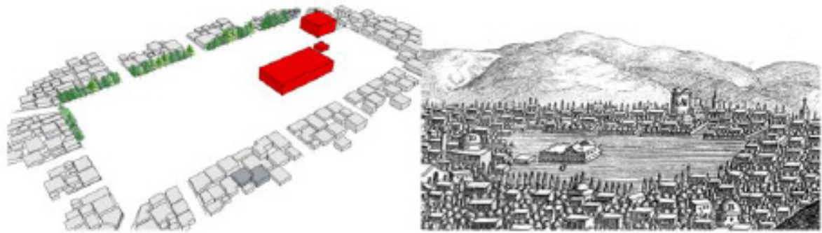
Fig. 7: The position of poplar trees in the south and west of the Saheb Abad square to reduce the effect of undesirable wind flow. Right fig: Chardin drawing of Saheb Abad square (Zoka, 1989, 51).
