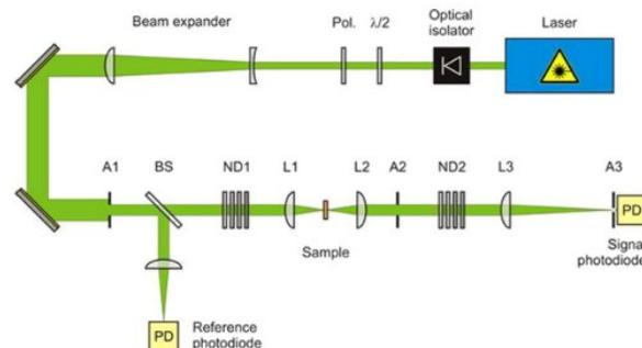
Figure 4. The closed Z-scan optical set up.
