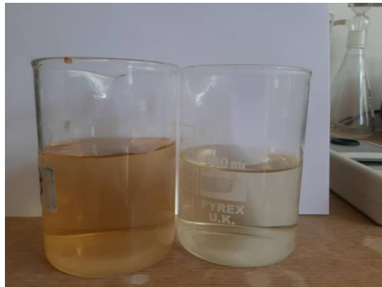
Fig 10. Effluent samples after biological treatment, before, and after ozonation
