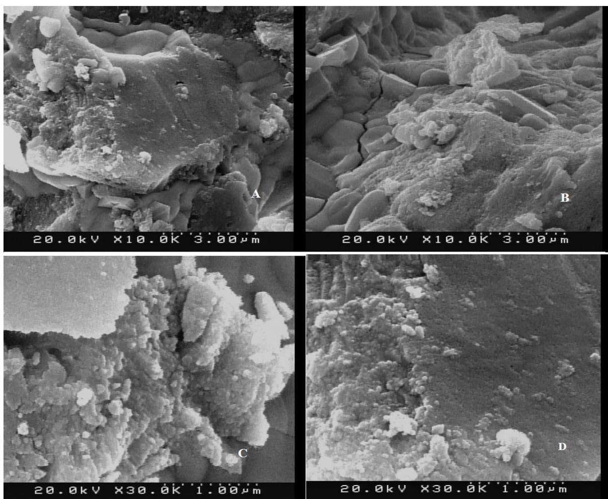
**Fig. 3.** FE-SEM images of NiO-SnO<sub>2</sub> (A, 50/50% Ni/Sn ratio), NiO-SnO<sub>2</sub> (B, 25/75% Ni/Sn ratio), NiO-SnO<sub>2</sub> (C, 10/90% Ni/Sn ratio), and NiO-SnO<sub>2</sub> (D, without use of grape extract)
