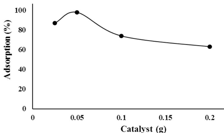
Fig. 8. Adsorption of Cd: effect of catalyst dosage (time: 90min; pH: 6.5; Cd: 40ppm; r.t.)
