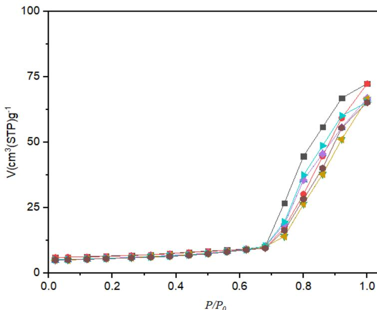
**Fig. 4.** N<sub>2</sub> adsorption- desorption isotherms of NiO-SnO<sub>2</sub> (1, 50/50% Ni/Sn ratio), NiO-SnO<sub>2</sub> (2, 25/75% Ni/Sn ratio), NiO-SnO<sub>2</sub> (3, 10/90% Ni/Sn ratio), and NiO-SnO<sub>2</sub> (4, without use of grape extract)
