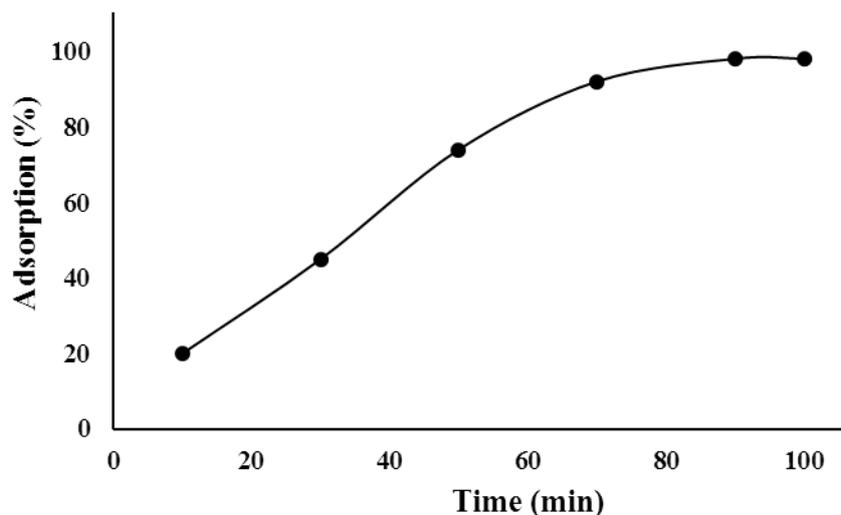
Fig. 6. Adsorption of Cd: effect of contact time (pH: 6.5; NiO-SnO<sub>2</sub>: 0.05g; Cd: 40ppm; r.t.)
