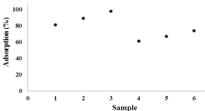
Fig. 7. Adsorption of Cd on the surface of NiO-SnO<sub>2</sub> (1, 10/90% Ni/Sn ratio), NiO-SnO<sub>2</sub> (2, 25/75% Ni/Sn ratio), NiO-SnO<sub>2</sub> (3, 50/50% Ni/Sn ratio), NiO (4), SnO<sub>2</sub> (5), and NiO-SnO<sub>2</sub> (6, without use of grape extract), (time: 90min; cat.: 0.05g; pH: 6.5; Cd: 40ppm; r.t.)
