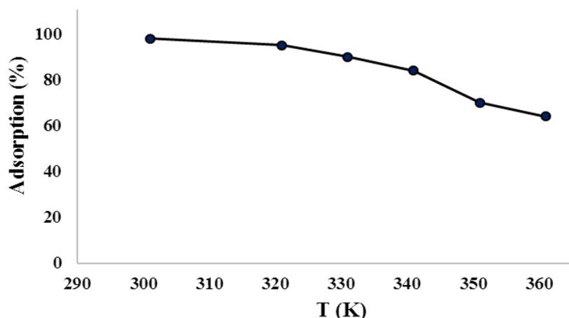
**Fig. 11.** Adsorption of Cd: effect of temperature (time: 90min; cat.: 0.05g; Cd concentration: 40 ppm; pH: 6.5; r.t.)
