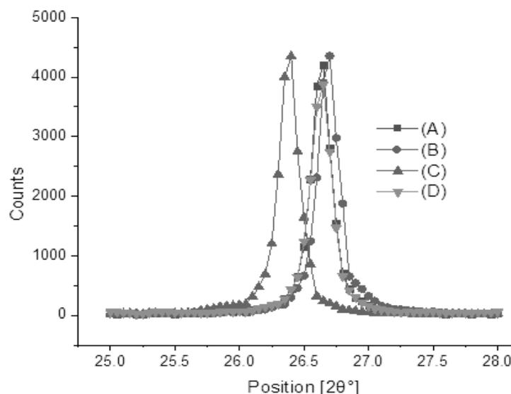
**Fig. 2.** Changes on the peak position of NiO–SnO<sub>2</sub> (A, 50/50% Ni/Sn ratio), NiO–SnO<sub>2</sub> (B, 25/75% Ni/Sn ratio), NiO–SnO<sub>2</sub> (C, 10/90% Ni/Sn ratio), and NiO–SnO<sub>2</sub> (D, without use of grape extract),
