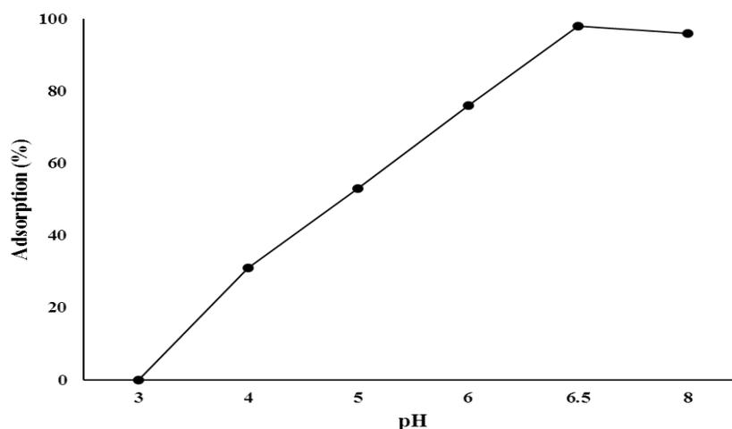
**Fig. 5.** Adsorption of Cd: effect of pH (time: 90min; NiO-SnO<sub>2</sub>: 0.05g; Cd: 40ppm; r.t.)
