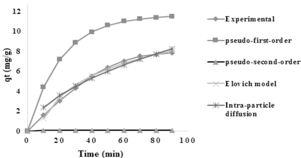
**Fig. 10.** Nonlinear adsorption rate curves (q<sub>t</sub> vs t) (Cd concentration: 40 ppm; cat.: 0.05g; pH: 6.5; r.t.)
