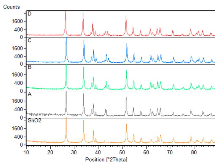
**Fig. 1.** XRD patterns of NiO–SnO<sub>2</sub> (A, without use of grape extract), NiO–SnO<sub>2</sub> (B, 50/50% Ni/Sn ratio of starting materials), NiO–SnO<sub>2</sub> (C, 25/75% Ni/Sn ratio of starting materials), NiO–SnO<sub>2</sub> (D, 10/90% Ni/Sn ratio of starting materials)
