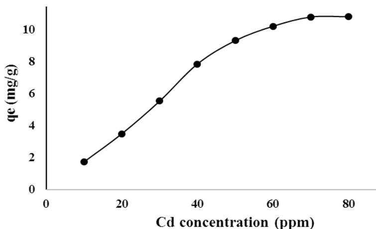
Fig. 9. Adsorption of Cd: effect of initial Cd concentration (time: 90min; cat.: 0.05g; pH: 6.5; r.t.)
