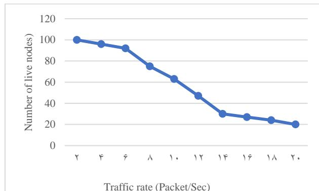
Fig. 5. Number of live nodes at different traffic rates
