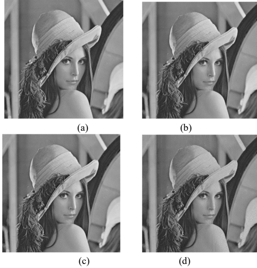
Fig.4. CS reconstructed image Lena with 10% measurement ratio. (a) SBCS-PL (PSNR=46.3 dB), (b) SBCS-IST (PSNR=34.43 dB), (c) SBCS-SPL (PSNR=47.6 dB), (d) SBCS-SIST (PSNR=50.8 dB).
