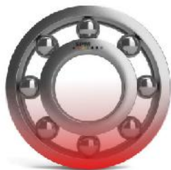
Fig. 6. A bearing with a downward-directed load zone (indicated by the transparent red area).
