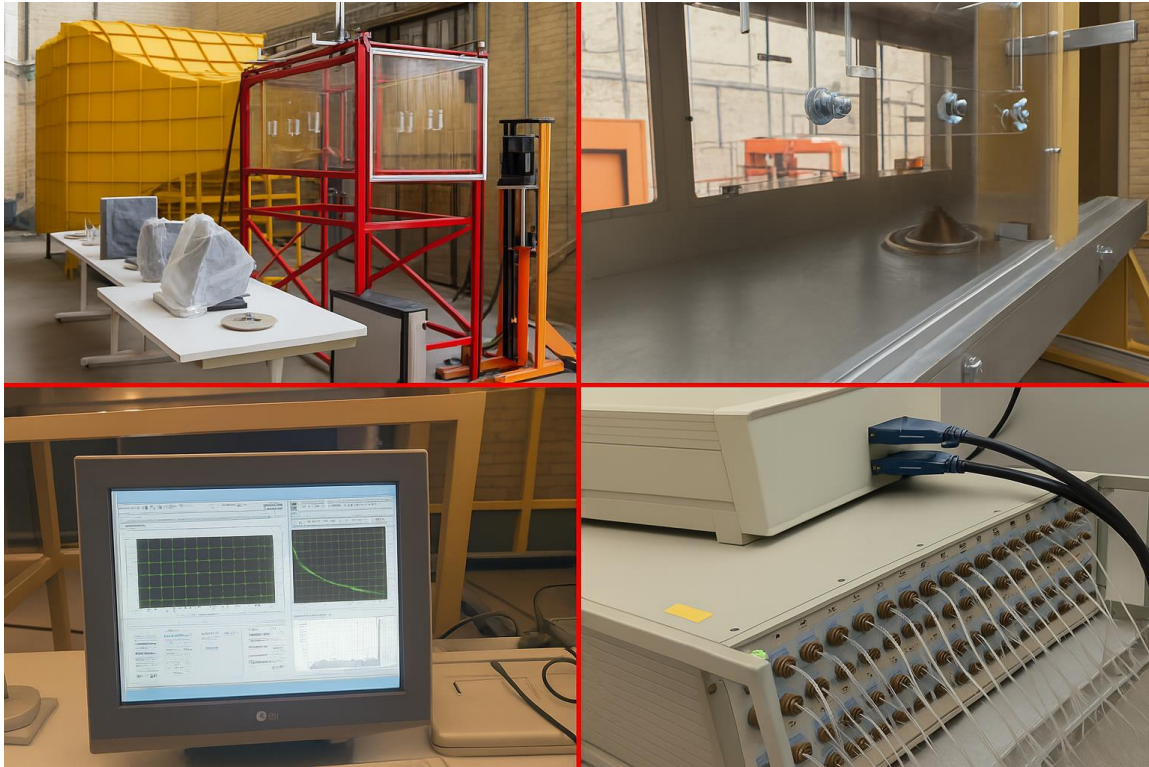
Fig. 4 The placement of domes in the wind tunnel, tunnel equipment, sensors, and analytical systems
