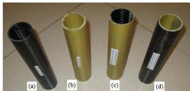
Fig 1. The specimens used in the study: carbon-only (a), Kevlar-only (b), Kevlar-outside/carbon-inside (c), and carbon-outside/Kevlar-inside (d)
