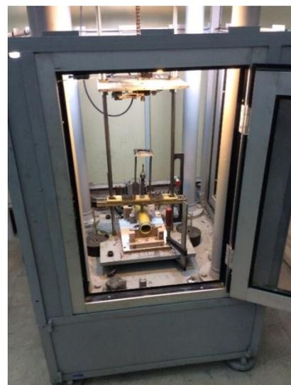
Fig 4. The drop-weight impact apparatus used in the study
