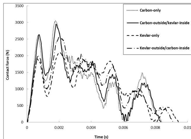
Fig 7. Experimental results for the contact force history of the specimens under study
