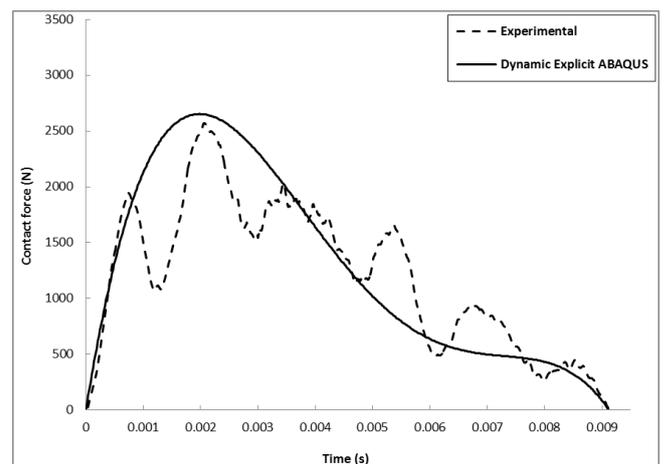
Fig 11. Experimental and numerical results for the contact force history of the Kevlar-outside/carbon-inside specimen.
