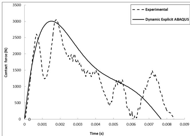
Fig 8. Experimental and numerical results for the contact force history of the carbon-only specimen.
