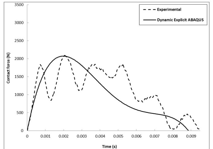
Fig 10. Experimental and numerical results for the contact force history of the Kevlar-only specimen.
