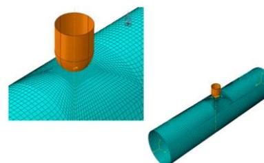
Fig 6. Modeling of the impactor using a rigid analytical shell and modeling of composite cylinders using the S4R element.
