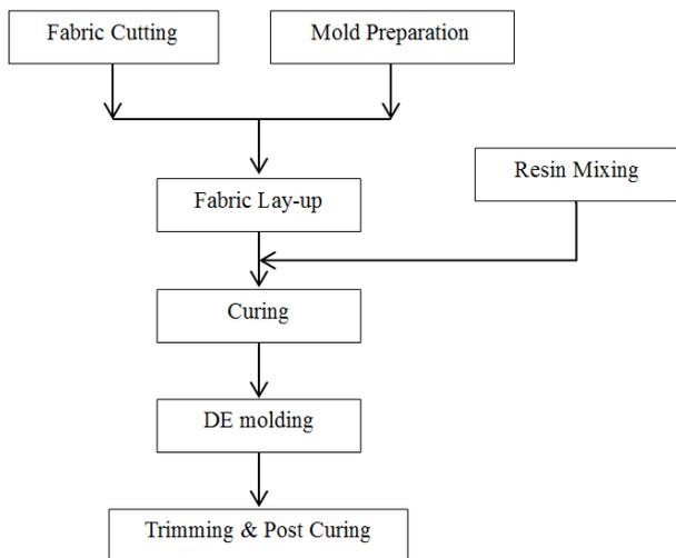
Fig 2. The manufacturing process of the specimens
