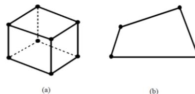
Fig 5. Continuum shell (SC8R) (a) and conventional shell (S4R) (b) elements.
