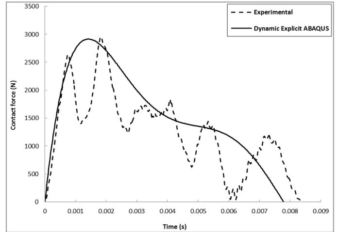
Fig 9. Experimental and numerical results for the contact force history of the carbon-outside/Kevlar-inside specimen.
