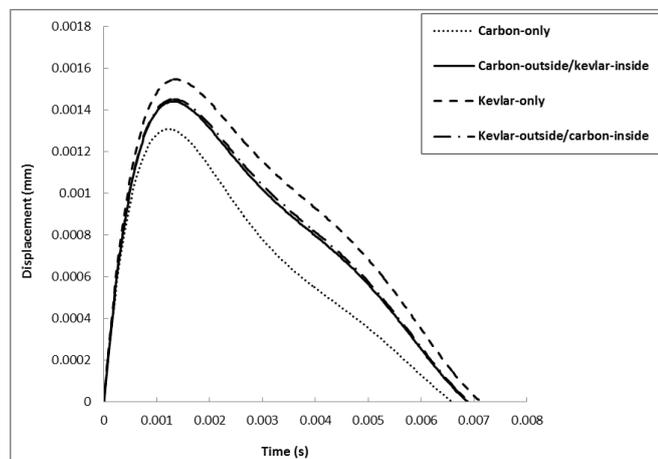
Fig 12. Numerical results for the deflection history of the specimens under study.
