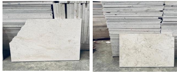
FIGURE 1 EXAMPLE OF CRACK DEFECT ON MARBLE SURFACE
