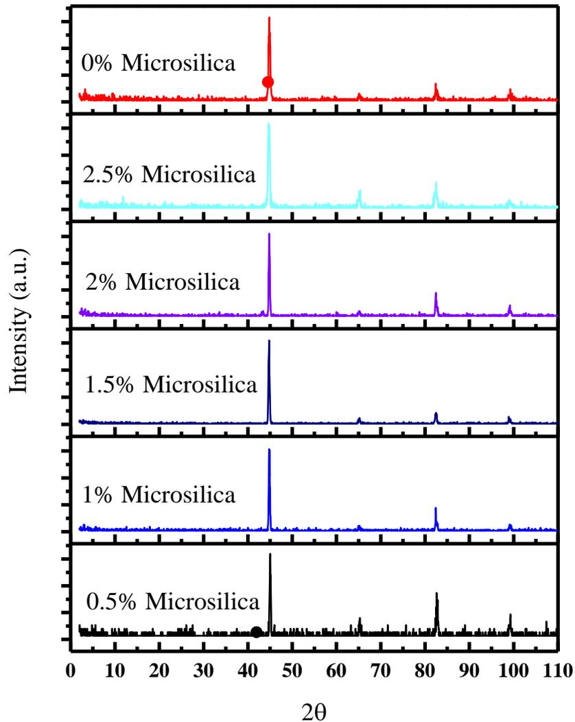
Fig. 4: X-ray diffraction pattern of ST35 steel samples welded in the presence of microsilica flux with percentages of 0, 0.5, 1, 1.5, 2 and 2.5 percent.
