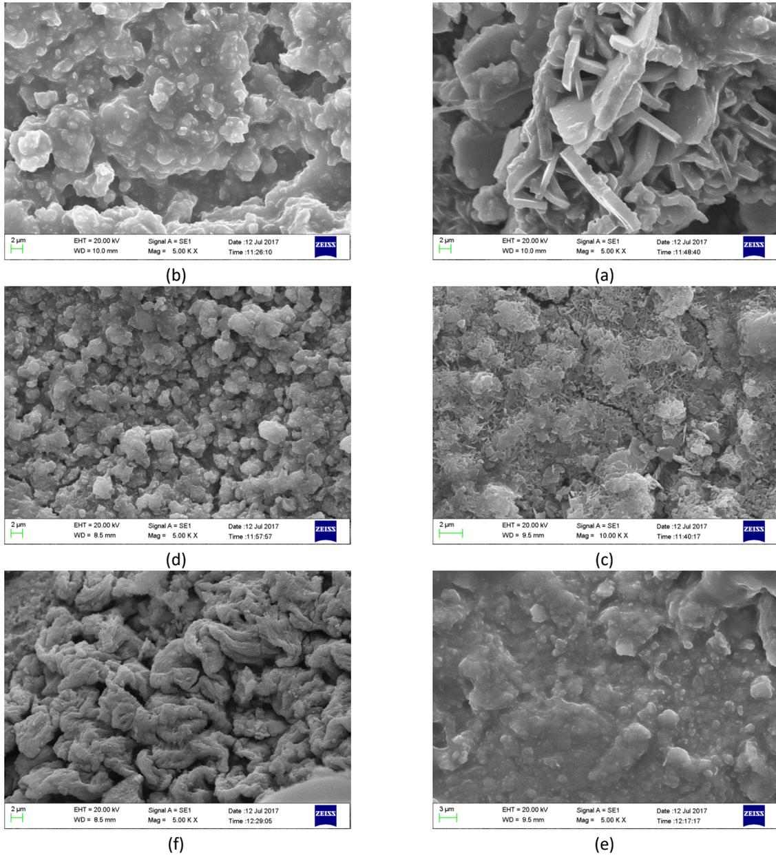
Fig. 3: Electron microscope images of the microstructure of the welded area of ST35 steel with different percentages of microsilica, a) 0.5%, b) 1%, c) 1.5%, d) 2%, e) 2.5%, and f) no microsilica.
