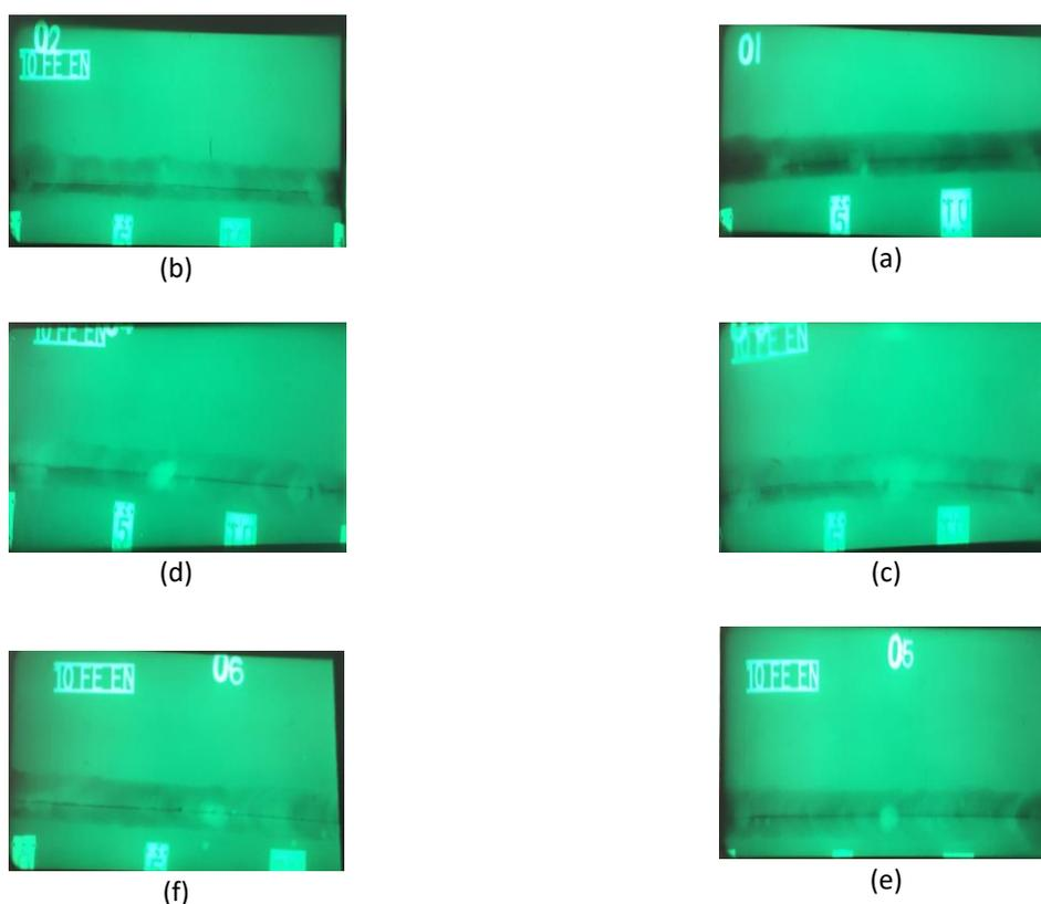
Fig. 1: Radiographic results of the welded area of ST35 steel with different percentages of microsilica, a) 0.5%, b) 1%, c) 1.5%, d) 2%, e) 2.5%, and f) no microsilica.
