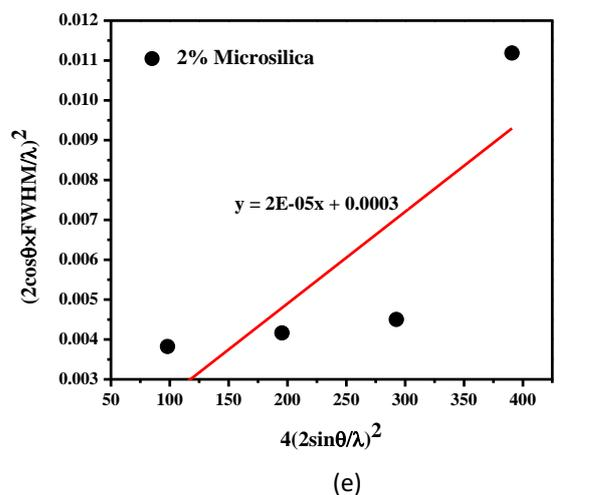
Figure 5 - Results from Williamson Hall analysis of ST35 steel samples welded in the presence of microsilica flux with percentages of 0, 0.5, 1, 1.5, 2 and 2.5 percent.
