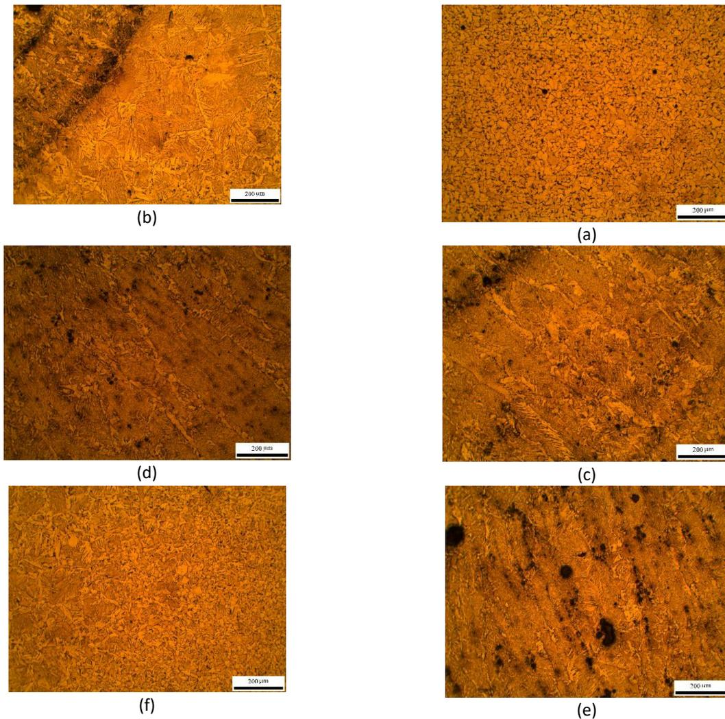
Fig. 2: Optical microscope images of the microstructure of the welded area of ST35 steel with different percentages of microsilica, a) 0.5%, b) 1%, c) 1.5%, d) 2%, e) 2.5%, and f) no microsilica.
