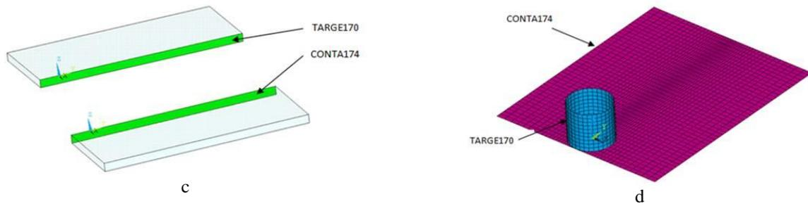
Fig. 3: a) Modeled image of the plates and welding pins, b) Meshed model, c) Surface-to-surface contact of target170 and conta174, and d) Surface-to-surface contact of target170 and conta174 between the plates and the tool
