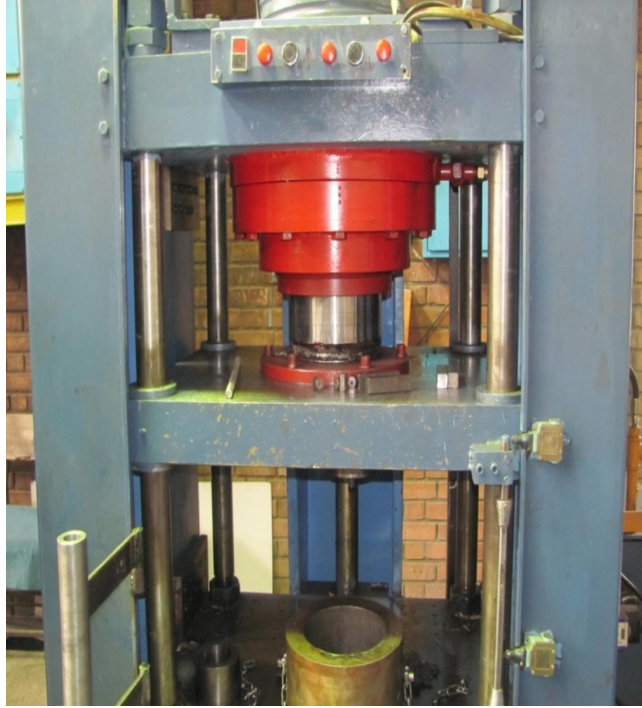
Fig. 3 40-ton hydraulic press used in experiments.
