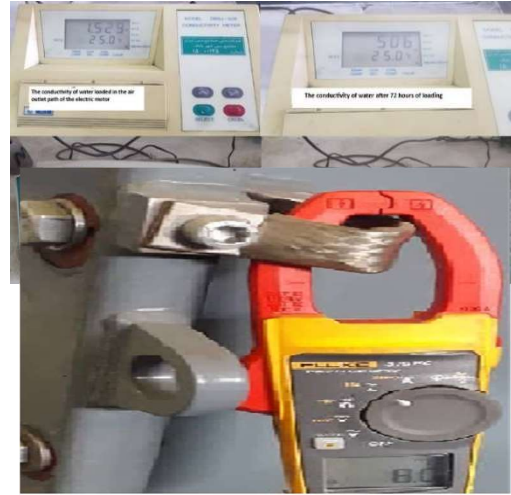
Figure 4: Examination of the electric motor grounding system and the presence of circulating currents
