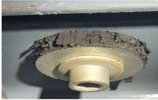
Figure 6: Presence of corrosion on the elastic rubber components
