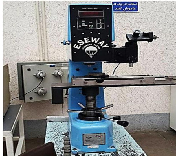
Fig. 2 The Vickers Hardness testing machine used for hardness measurement.
