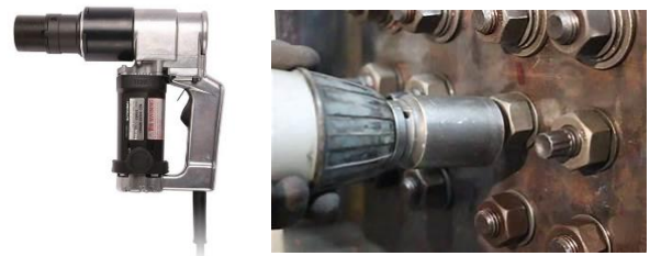
Fig 2. Electric shear wrench of TC bolts
