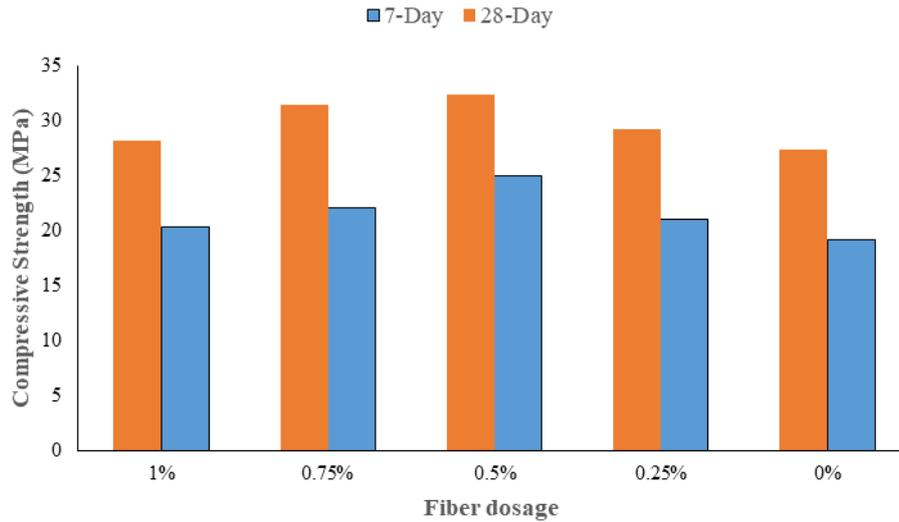
**Fig. 5. Effect of fiber dosage on compressive strength of concrete**
