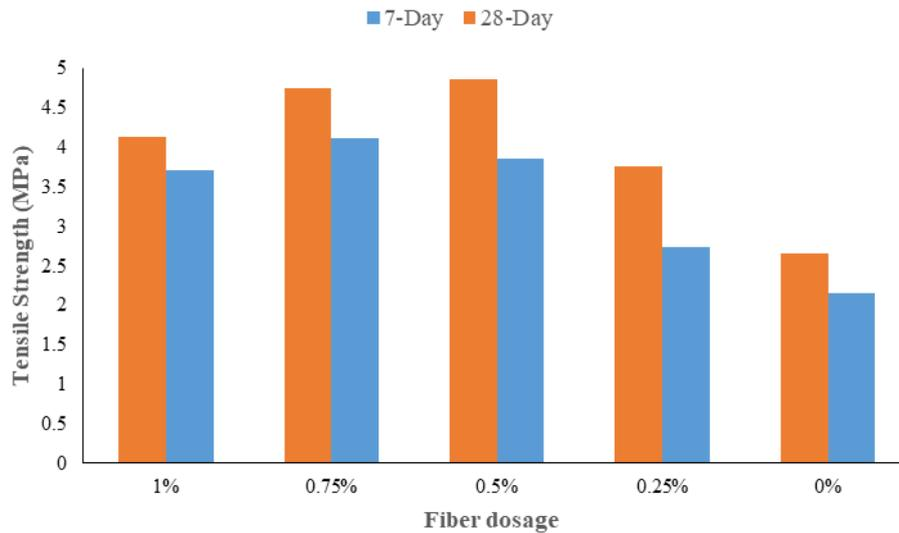
**Fig. 6. Effect of fiber dosage on tensile strength of concrete**
