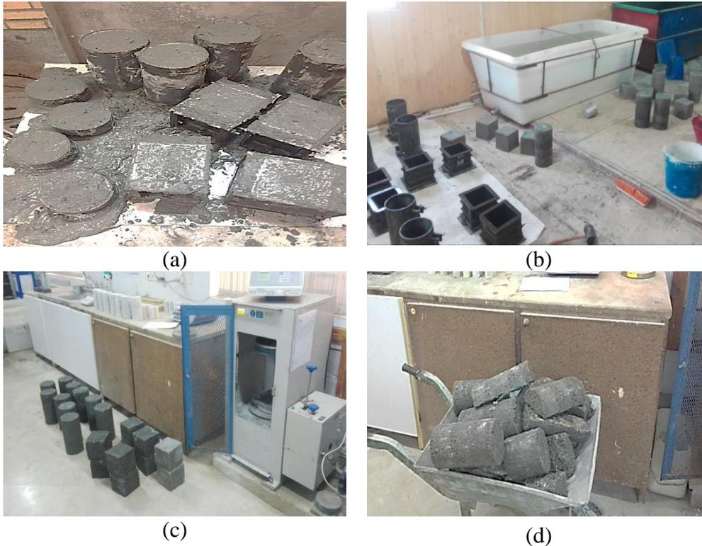
**Fig. 3. a) concrete placing in moulds, b) curing of samples, c) cylindrical and cubic samples before test, d) failure mode of cylindrical samples**
