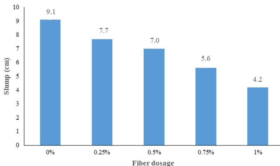
Fig. 4. Effect of fiber dosage on workability of fresh concrete
