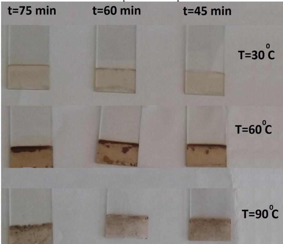
**Fig. 2.** Photograph of deposited layers at different growth time and temperatures.
