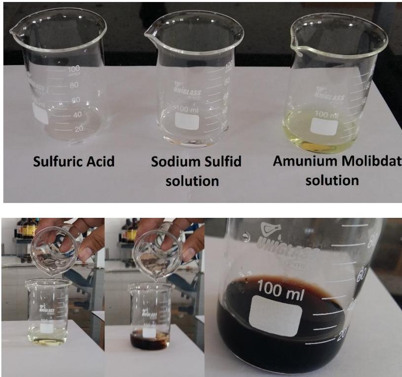
**Fig.1.** Progress of final solution production. Brown color of solution confirms presence of MoS<sub>2</sub>.
