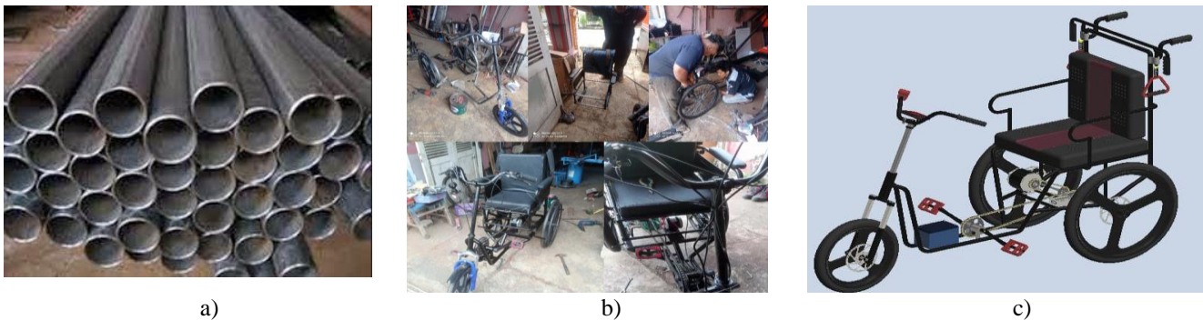
Fig. 1. a) Materials for designing a wheelchair frame, b) design process, and c) sketch of the final shape of a wheelchair for stroke sufferers
