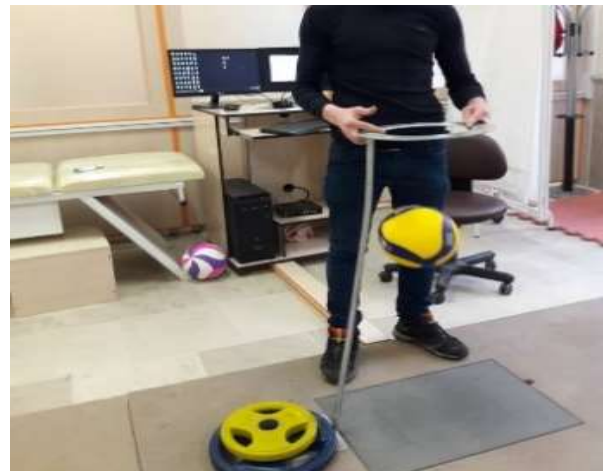
Fig. 5 Recording the GRFS using a device designed to reduce the measurement error.
