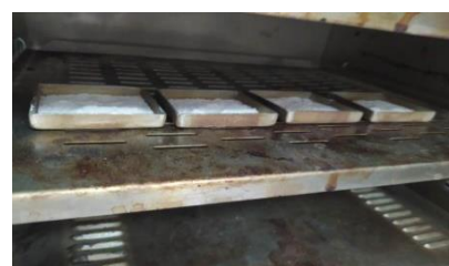
Fig. V. Technique for determining the water content of flours
