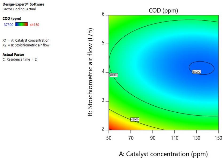
Fig. 5- Two-dimensional plot of the interaction between catalyst concentration and stoichiometric air flow on the COD response
