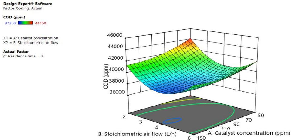
Fig. 6- Three-dimensional plot of the interaction between catalyst concentration and stoichiometric air flow on the COD response
