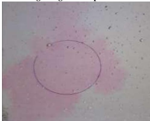
**Figure 5 - Experiment on the concrete surface color of the sample with 2.5% titanium dioxide after 24 hours. Comparison of Figure 4 and 5 shows that self - cleaning properties were significantly affected by Nano TiO<sub>2</sub>.**
