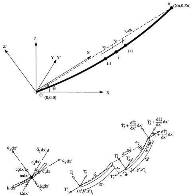
Fig. 1 the model of 3D cable for static analysis
