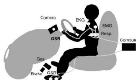
Fig. 1 How to connect the electrodes to the driver [21].
