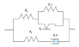
Fig.1. The two-layer viscoplasticity model [39]
