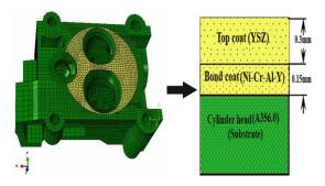
Fig. 2. The FE model of the coated cylinder head
