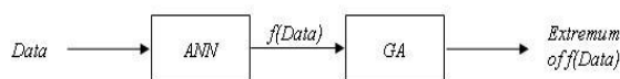
Fig. 3 The schematic diagram of using an artificial neural network and genetic algorithm for the extremum determination of a set of data
