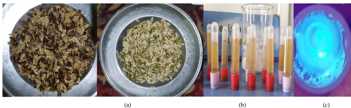
Figure 1. (a) Pumpkin seed precursor (b) Carbon dots under visible light (c) Carbon dots under UV light.
