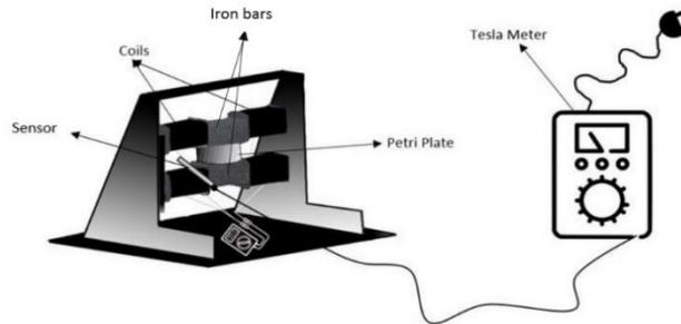
Figure 1. The experimental electromagnet setup (Naz *et al.*, 2012)
