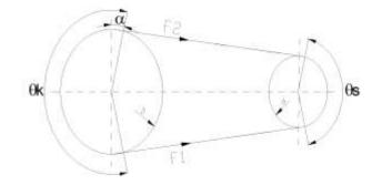
Fig.3. Applied forces on both sides of belt in a pulley-belt transmission system
