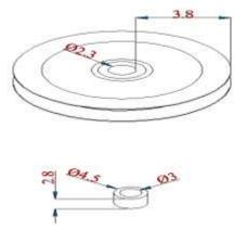
Fig.12. schematic diagram of abrasive brush with dimension of filler bush
