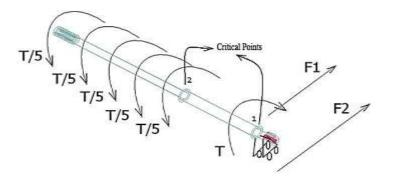
Fig.9. Diagram of bending moment of shaft and it's torque
