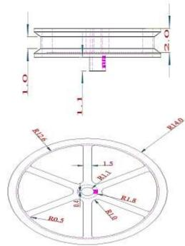
Fig.4. Driven pulley
