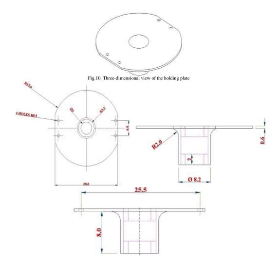
Fig.11. Blue print of holding plate
