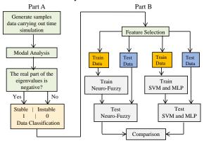
Fig. 4. Dynamic Simulation of system and training procedure
