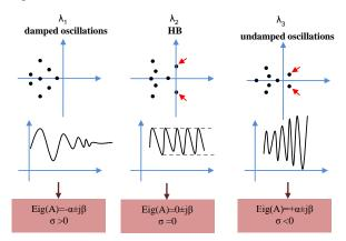
Fig. 1. Relation between the critical eigenvalues of dynamic algebraic Jacobian and power system oscillations
