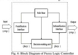
The fuzzification step involves taking a crisp input, such as the change in the voltage reading, and combining it with stored membership function to produce fuzzy inputs. To transform the crisp inputs into fuzzy inputs, membership function must be first assigned for each input. Once the membership functions are assigned, fuzzification take a real time inputs and compares it with the stored membership function information to produce fuzzy input values.
