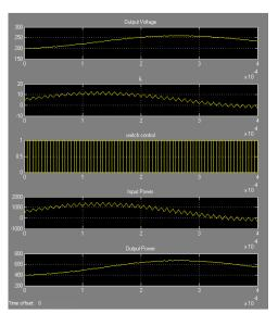
Fig.13. Module voltage, inductor current, switch control, and input and output power, the settling time of  $4 \times 10^{-3}$ .
