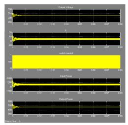
Fig.11. Module voltage, inductor current, switch control, and input and output power, the settling time of 0.08.
