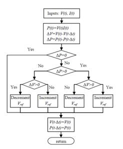
Fig 2. Flow chart for P&O algorithm [10].
