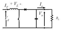
Fig. 5: The Boost converter circuit.
