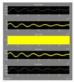
Fig 12. Module voltage, inductor current, switch control, and input and output power, the settling time of  $3 \times 10^{-3}$ .
