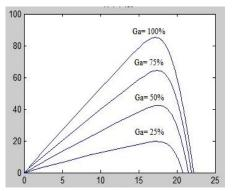
Fig3. P-V curves under changing the solar radiation.
