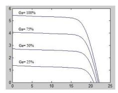
Fig4. I-V curves under changing the solar radiation.
