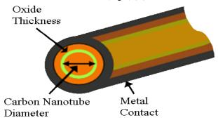
Fig.1. Optimized geometry assumed for CNTFETToy.
