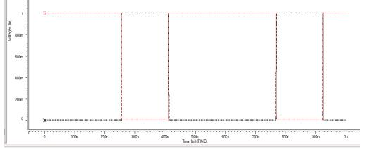
Fig.7. The input-output signals for ANN CNTFET inverter.
