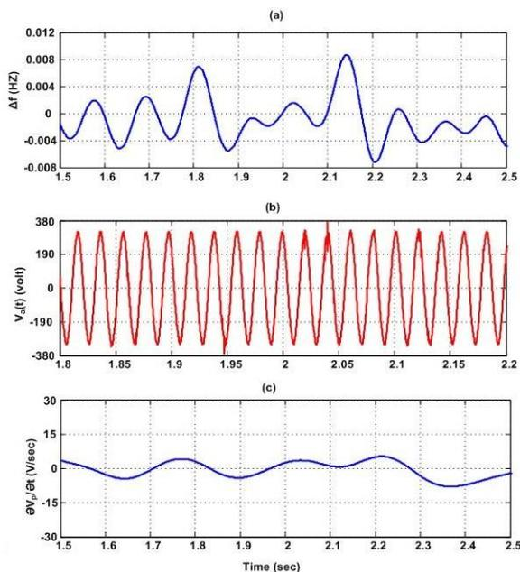
Fig 15: dynamic response of experimental system, a) frequency deviation of PCC voltage b) instantaneous voltage c) rate of change of positive sequence of voltage
