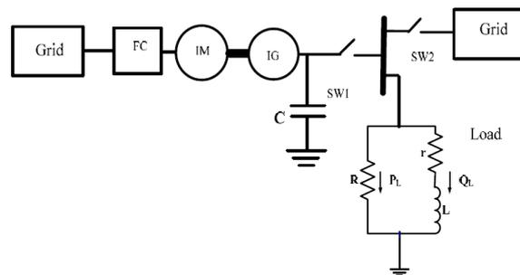
Fig 2.single line diagram of implementation system in order to islanding condition detection
