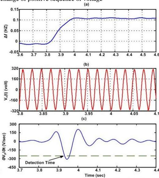
Fig 9: dynamic response of experimental system, a)frequency deviation of PCC voltage b) instantaneous voltage c) rate of change of positive sequence of voltage
