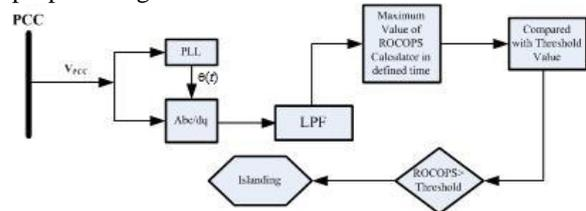
Fig 7. Proposed algorithm in order to islanding detection
