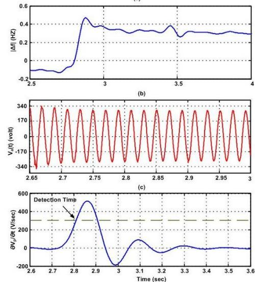
Fig 11: dynamic response of experimental system, a) frequency deviation of PCC voltage b) instantaneous voltage c) rate of change of positive sequence of voltage
