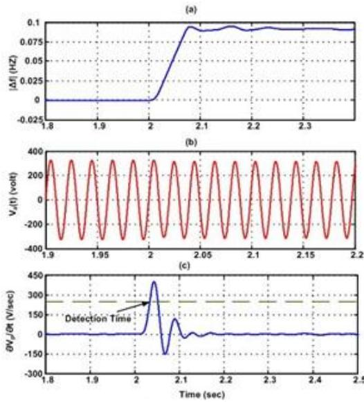
Fig 8: dynamic response of simulation system, a)frequency deviation of PCC voltage b) instantaneous voltage c) rate of change of positive sequence of voltage
