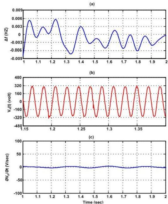
Fig 13: dynamic response of experimental system, a) frequency deviation of PCC voltage b) instantaneous voltage c) rate of change of positive sequence of voltage
