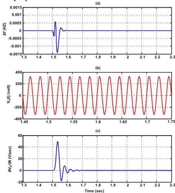
Fig 12: dynamic response of simulation system, a) frequency deviation of PCC voltage b) instantaneous voltage c) rate of change of positive sequence of voltage
