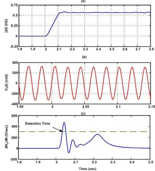
Fig 10: dynamic response of simulation system, a) frequency deviation of PCC voltage b) instantaneous voltage c) rate of change of positive sequence of voltage
