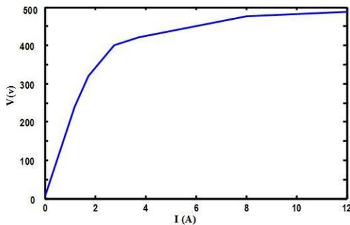
Fig 4. Motor and Generator saturation curves.
