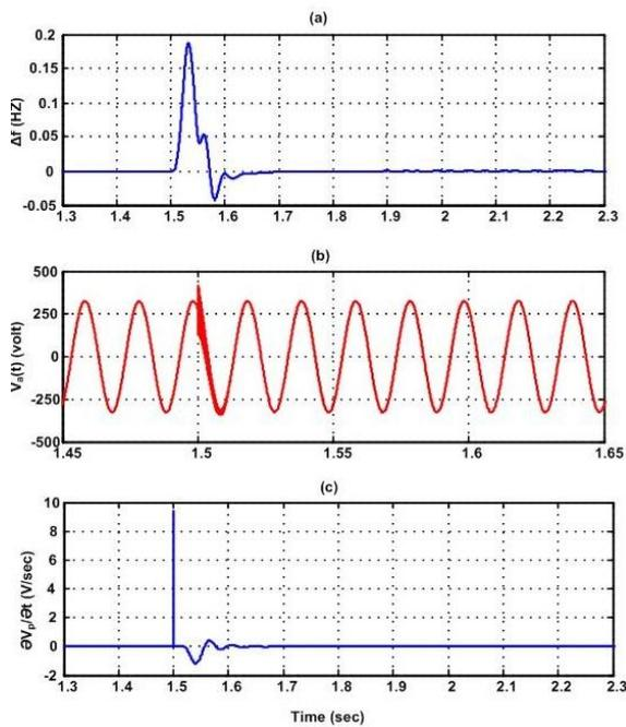
Fig 14: dynamic response of simulation system, a) frequency deviation of PCC voltage b) instantaneous voltage c) rate of change of positive sequence of voltage
