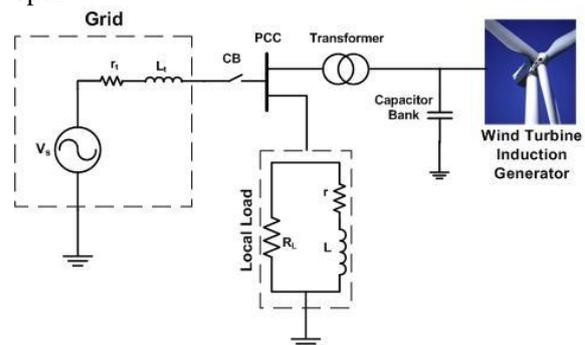
Fig.1. Single line diagram of study system
