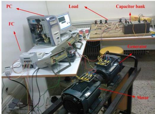
Fig 3: Implementation system in order to islanding condition detection
