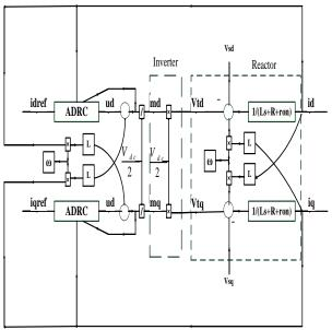
Fig. 4. Current loop structure of ADRC in dq-frame
