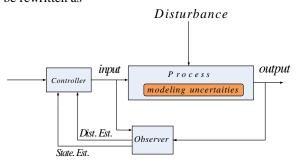
Fig. 1. Simplified block diagram of ADRC for a process
