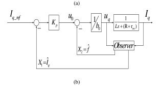
Fig. 5. Simplified block diagram of current loop of ADRC (a) d-axis (b) q-axis
