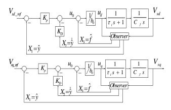
Fig. 8. Simplified block diagram of voltage loop of ADRC (a) d-axis (b) q-axis
