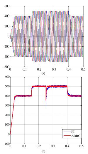
Fig. 9. Voltage of three phase inverter (a) three phase voltage (  $V_{sabc}$  ) (b) voltage in d- axis (  $V_{sd}$  )
