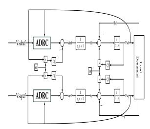
Fig. 7. Voltage loop structure of ADRC in dq-frame
