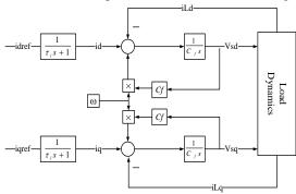
Fig. 6. Load voltage dynamics by considering equivalent system of current loop
