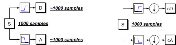
Fig. 3. Single-Stage Wavelet Transform with down sampling process [3]
