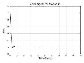
Fig.12. Error signal after controller design with second fitness function
