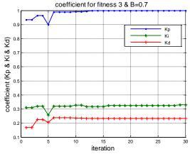
Fig.16. PID controller parameters convergence with third fitness function,  $B{=}0.7$
