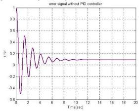
Fig.10. Error signal before controller design
