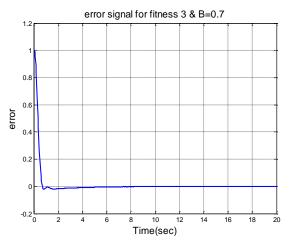
Fig.13. Error signal after controller design with third fitness function,  $B\!=\!0.7$
