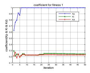
Fig.14. PID controller parameters convergence with first fitness function
