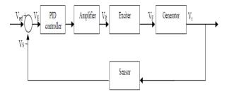
Fig.2. AVR system block diagram along with PID controller
