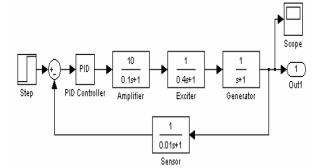
Fig.3.The block diagram of AVR system
