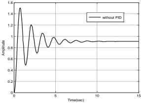
Fig.4. Output voltage step response without PID controller
