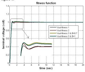
Fig.5. System output voltage step response with PID controller
