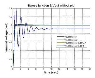
Fig.6. Comparison of output voltage step response before and after employing PID controller
