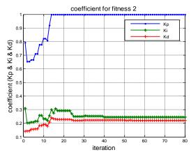
Fig.15. PID controller parameters convergence with second fitness function
