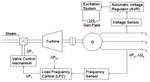
Fig.1. AVR and LFC system diagram
