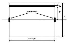
Fig. 1. The surface of the lightning strike to the ground [12]
